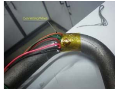
Fig. 4 : Rectangular strain-rosette with connecting wires
