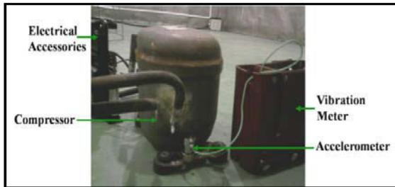
Fig. 12 : Experimental Setup of Vibration Measurement
