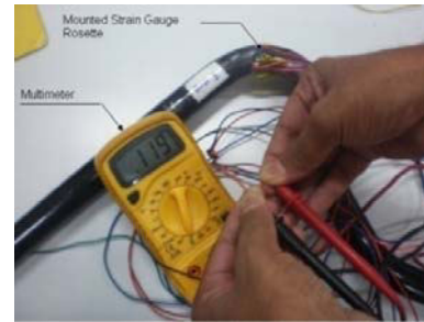
Fig. 5 : Checking of gauge resistance for gauge continuity
